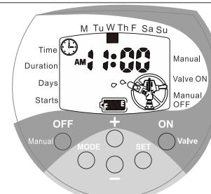
Used to shut-down time in winter or when it is not needed. Set schedules will be retained. You must turn this feature off to resume programmed watering schedules.
