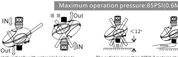
Install vertically with water inlet on top to prevent water from entering from the bottom
